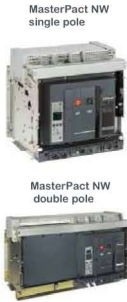
NW3213D2EM MasterPact NW32, H1 type (Icu = Ics = 65 kA), 3 poles, Drawout type, Micrologic 2.0E, Horizontal rear connections.
